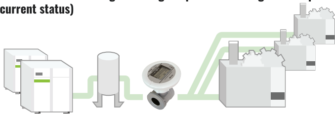
Flowmeter installed behind receiver tank
